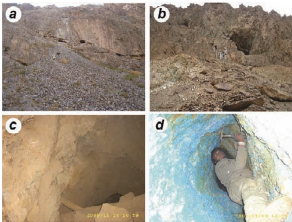
Figure 4A-9. Photographs of underground and surface workings in the Balkhab copper prospect area. (a) Narrow workings dipping into the hillside following schistosity and bedding in the host rocks. (b) Local “glory holes” sunk into the mineralized zones along the hillside. (c) Interior of a shaft inside the mine workings. (d) Narrow crawl hole excavated along malachite-rich zone. Photographs by Abdul Gaffer, Afghanistan Geological Survey.
