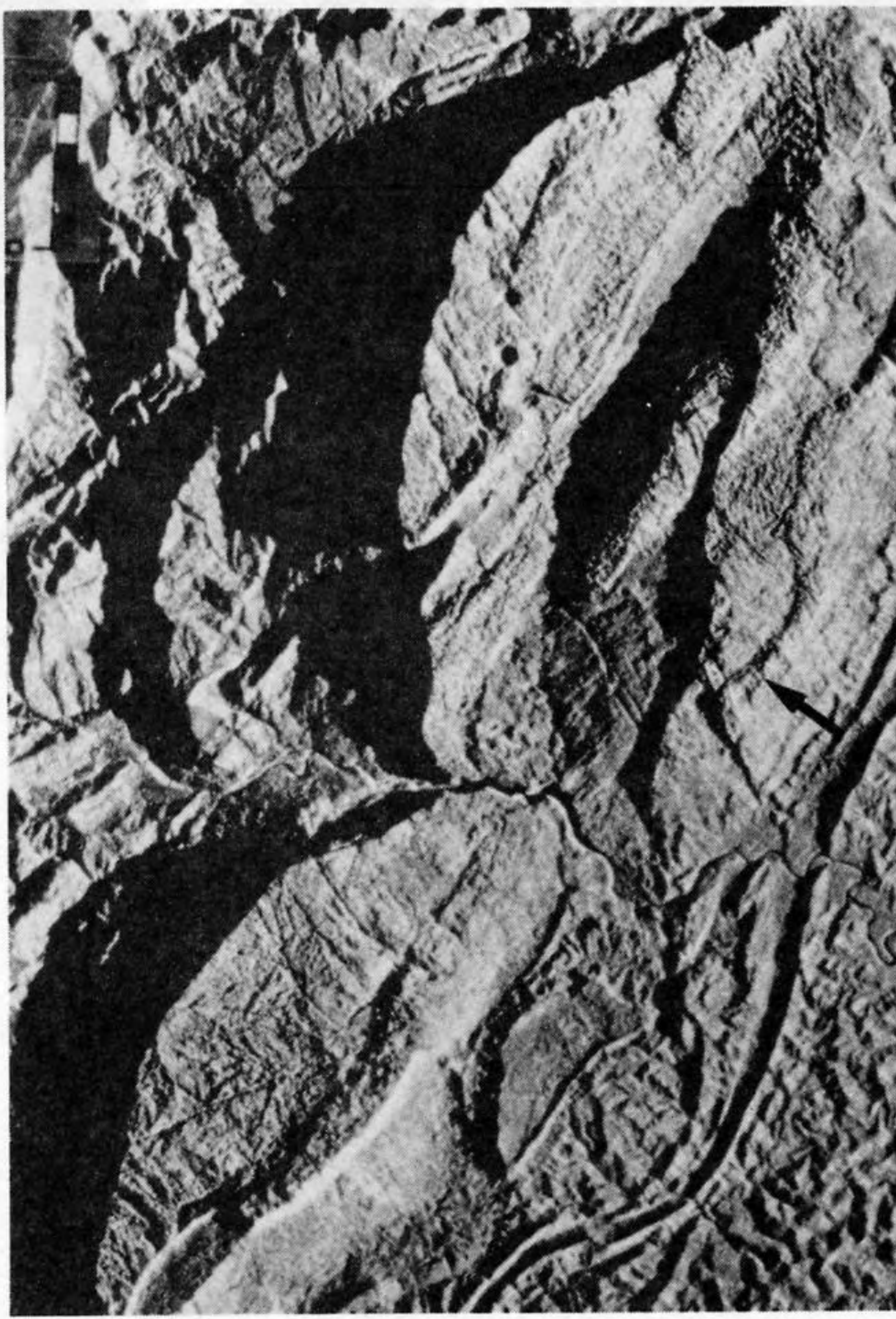
Figure 7. SAR stereopair (A and B) compared for geological information with same-scale plots of the Landsat MSS image (C) and published geologic map (D). The near-range portion of flight strip (B) has more terrain illuminated than the mid-range image (A) due to the steeper depression angle of the radar beam. Two unmapped anticlines are clearly seen on SAR (arrow on A). The SAR imagery has the most structural and karst information.
