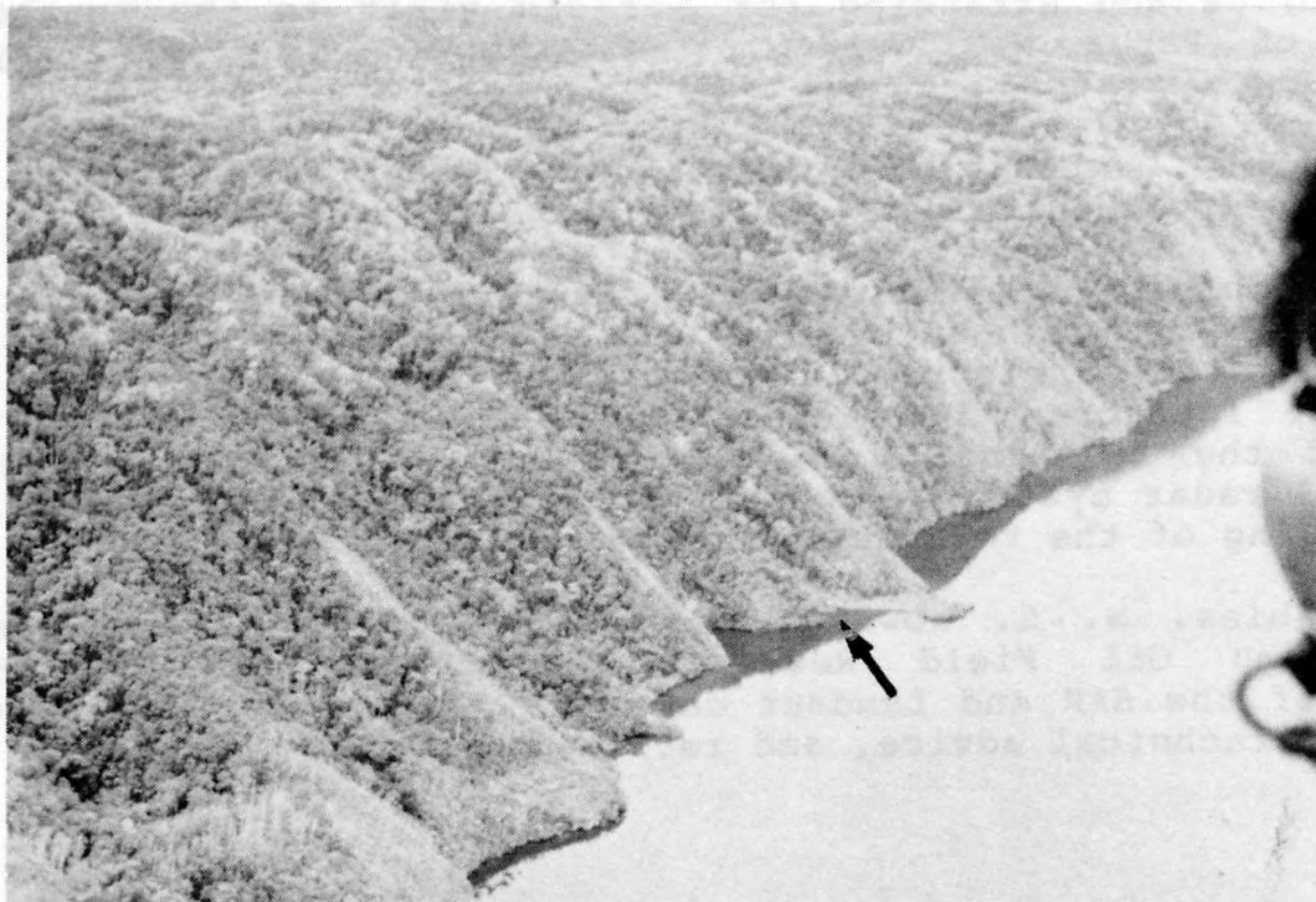
Figure 2. Darai Limestone dips steeply on the flank of Kutubu anticline. Small huts can be seen along the shoreline for scale. Topographic relief from lake to crest of anticline is 500 m. Rugged karst topography has developed on the limestone, making seismic technology impractical.
