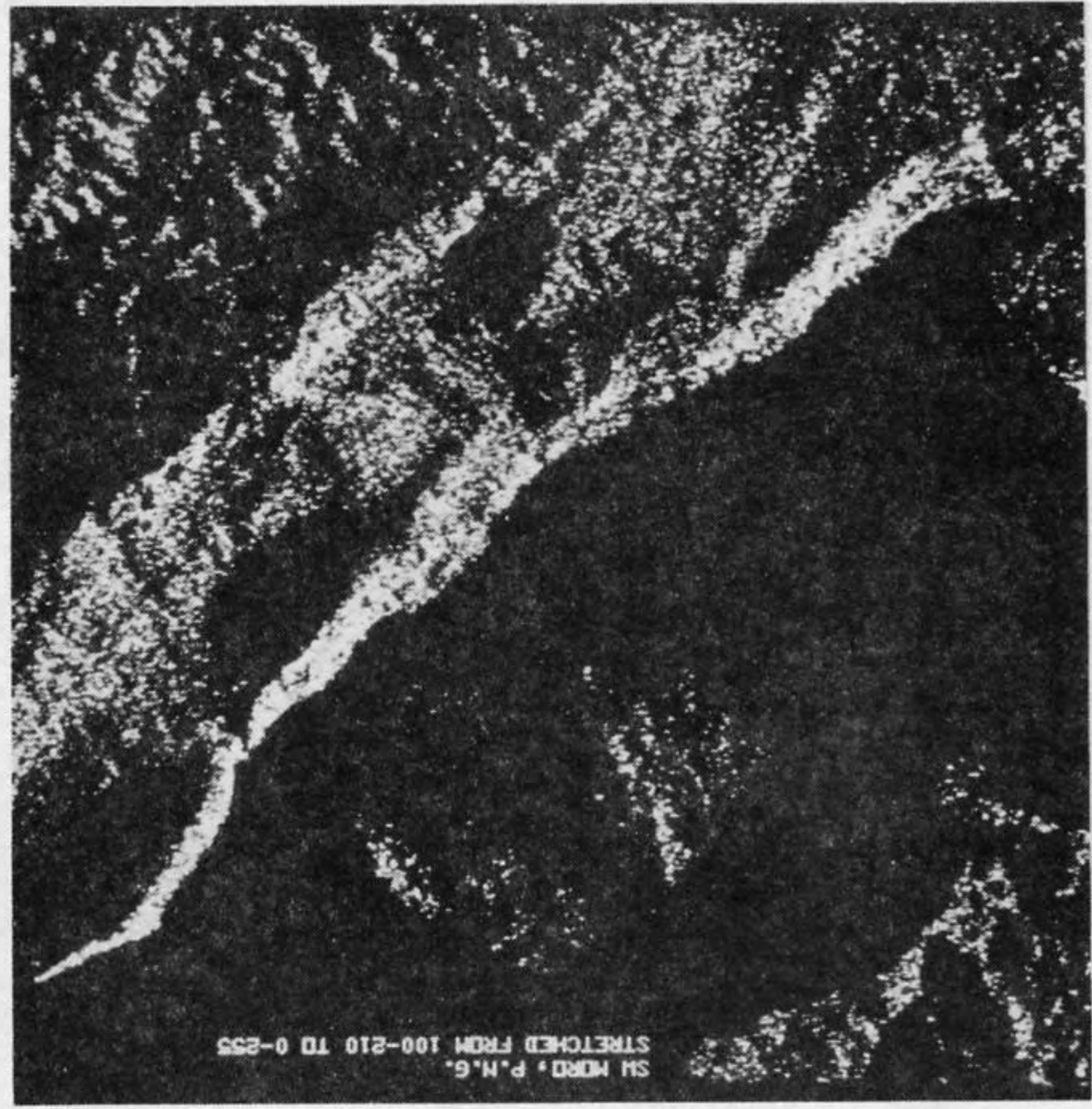
Figure 15. Digital reprocessing (contrast stretching) of SAR subscene (B) obtained from oversaturated (bright) cliffs that faced the radar antenna. This contrast stretching degraded (as expected) the rest of the scene (see Section 10.0).
