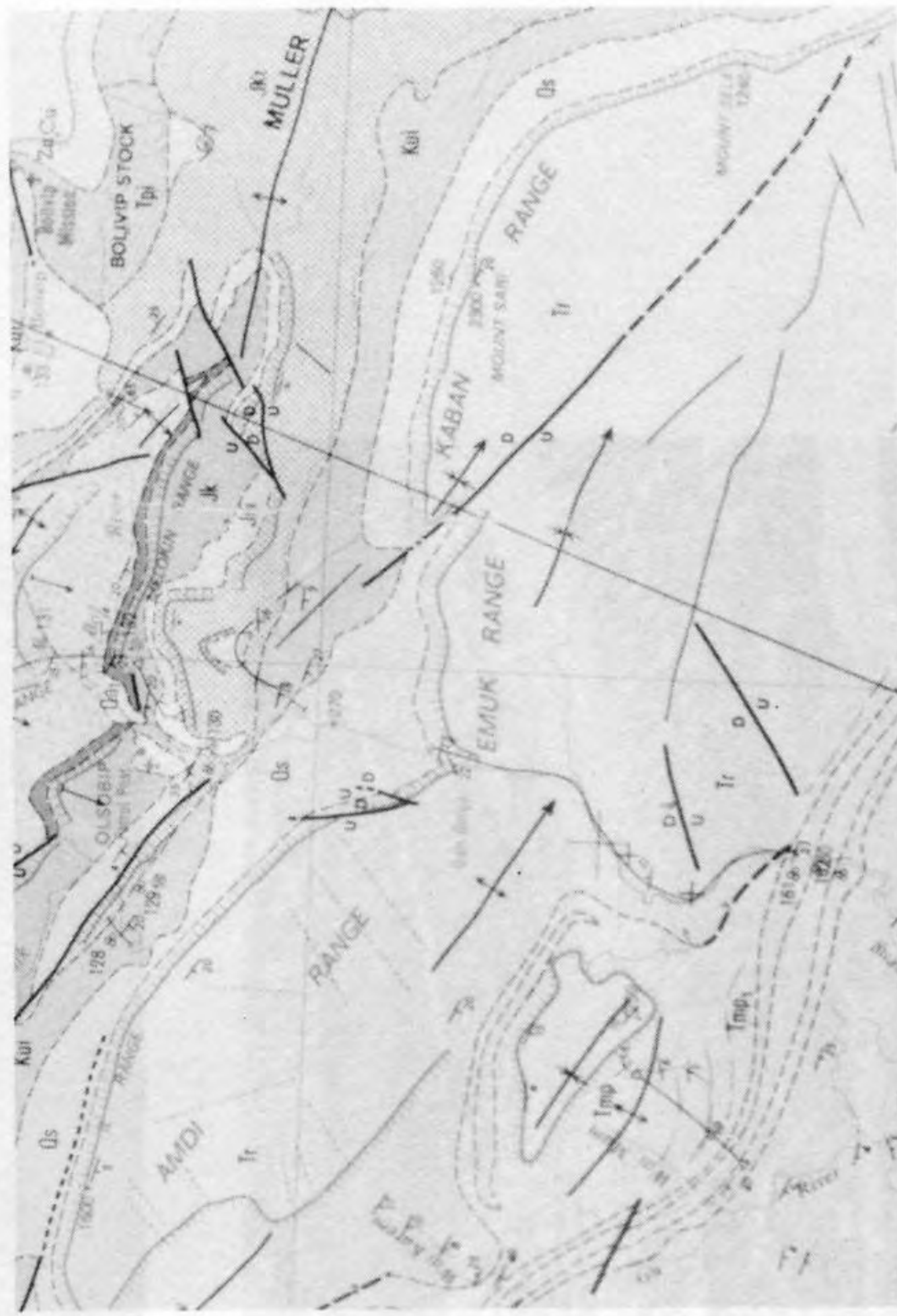
Figure 7. SAR stereopair (A and B) compared for geological information with same-scale plots of the Landsat MSS image (C) and published geologic map (D). The near-range portion of flight strip (B) has more terrain illuminated than the mid-range image (A) due to the steeper depression angle of the radar beam. Two unmapped anticlines are clearly seen on SAR (arrow on A). The SAR imagery has the most structural and karst information.
