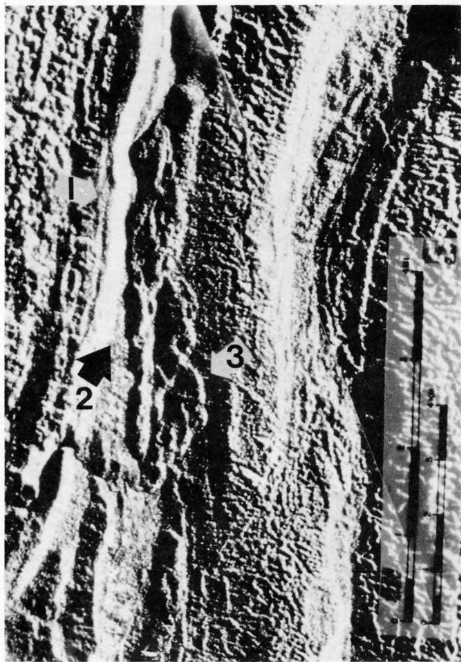
Figure 6. Comparison of radar image with color photo of a (1) thrust fault carrying Darai Limestone over shales, (2) stratigraphic contact between shales and resistant limestone, and (3) outcrop pattern of Darai strata folded into an anticline. Pitted and irregular radar signature of deeply weathered limestone contrasts with smooth, medium-gray signature of shales.
