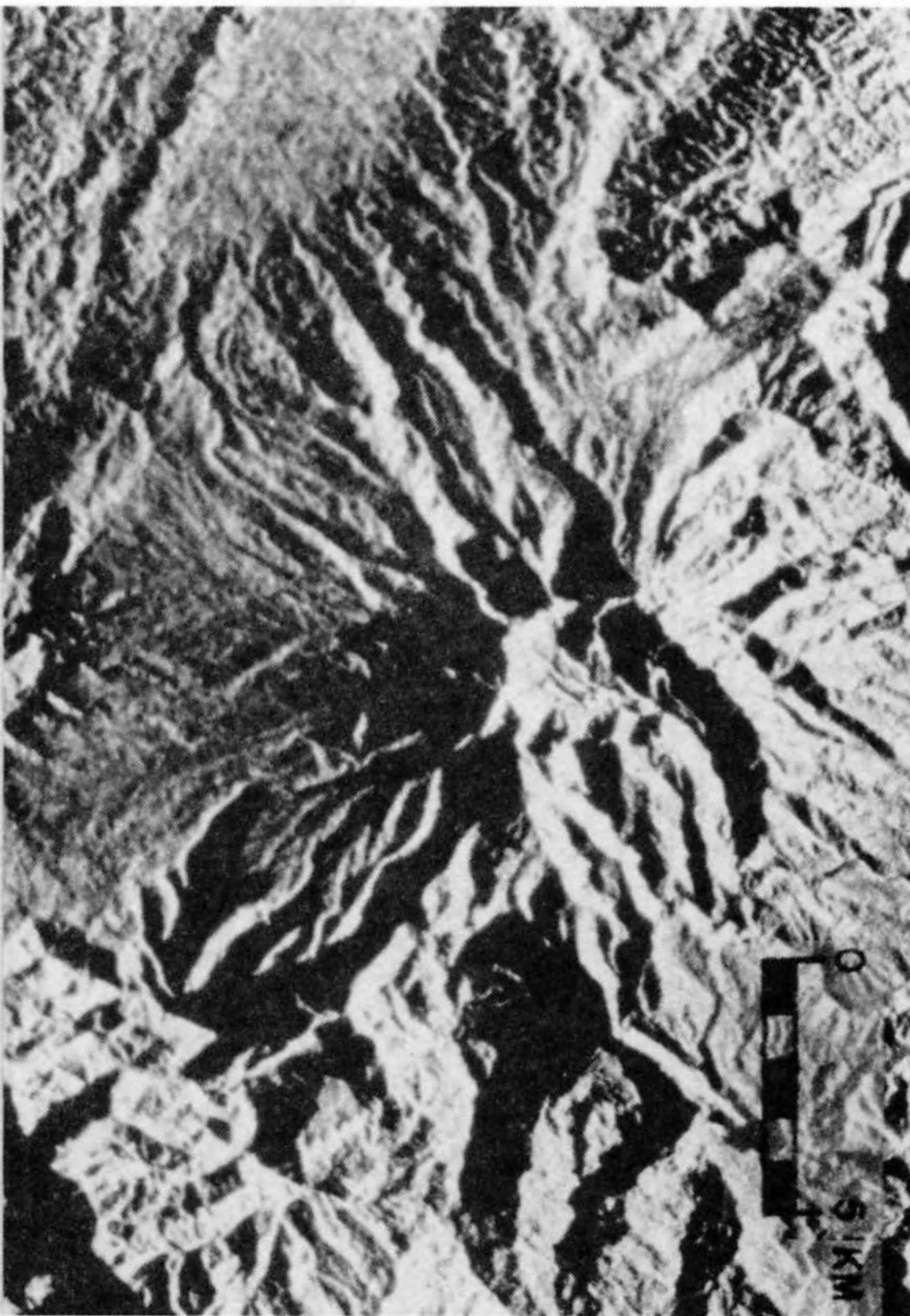
Figure 8. Suspected faults mapped on the geologic sheet as trending NW-SE through craters can be expanded upon with SAR. SAR shows valleys that trend NE-SW as deeply eroded into flanks of Mt. Sisa, suggesting a major zone of structural weakness.
