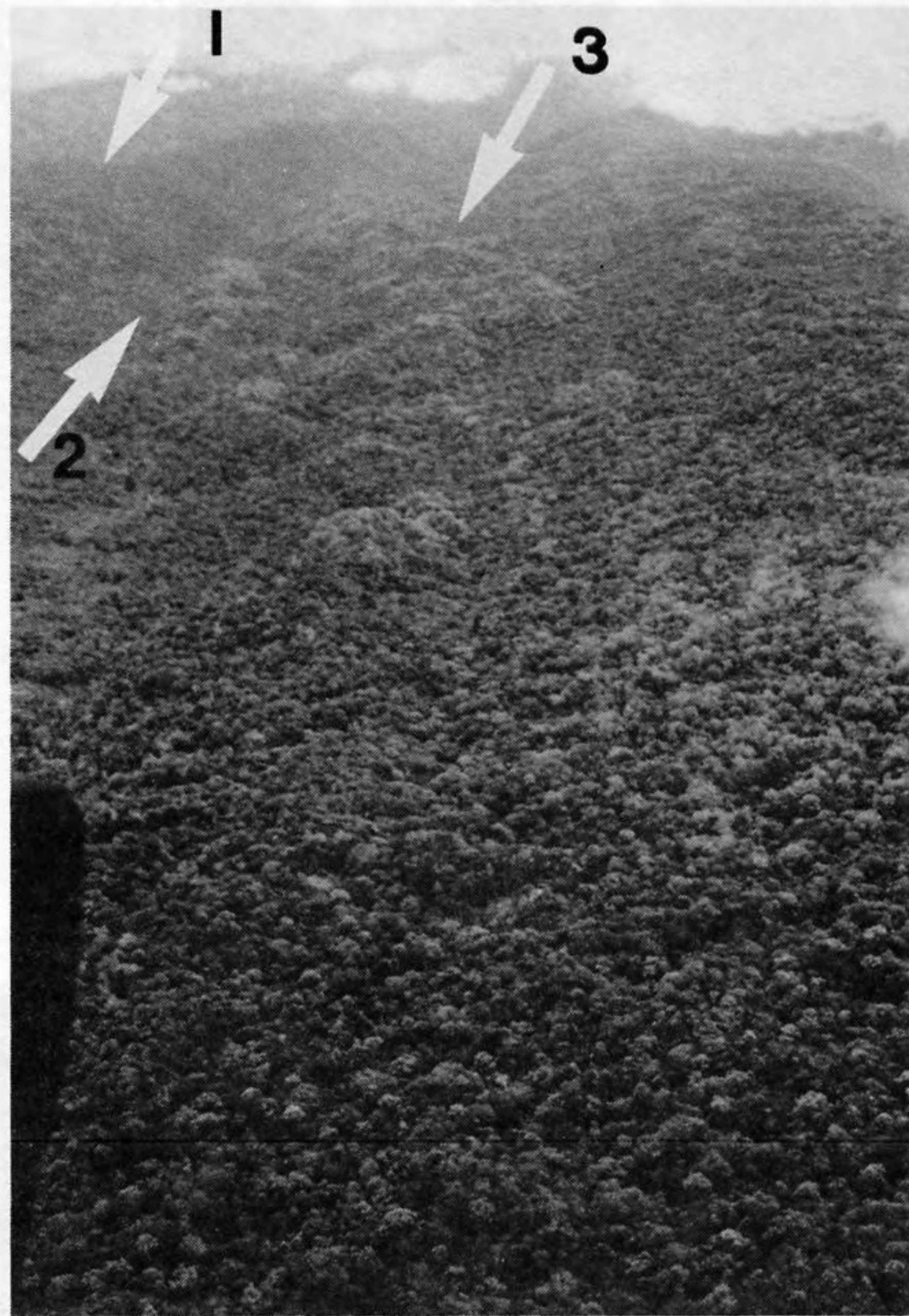
Figure 6. Comparison of radar image with color photo of a (1) thrust fault carrying Darai Limestone over shales, (2) stratigraphic contact between shales and resistant limestone, and (3) outcrop pattern of Darai strata folded into an anticline. Pitted and irregular radar signature of deeply weathered limestone contrasts with smooth, medium-gray signature of shales.
