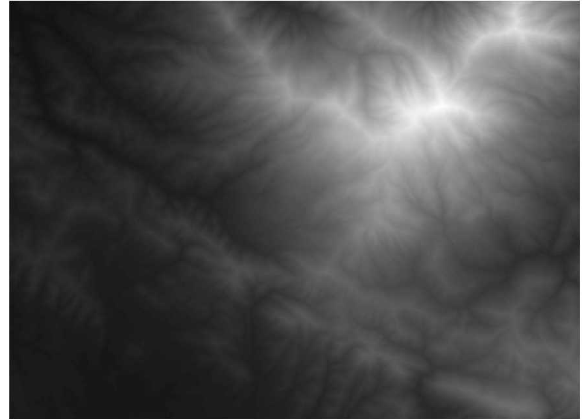
10-m USGS DEM where Light Tones are High and Dark Tones are Low
