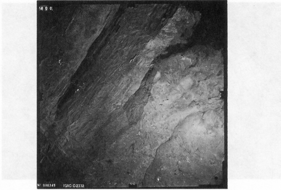
Figure 9. Typical aerial photograph of Sumapaz area showing detailed topography. Interpreted with stereoscope for quantitative strike and dip determination.
