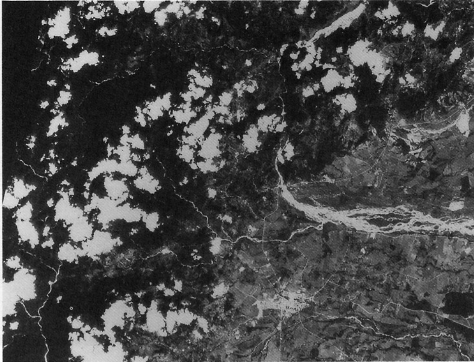
Figure 13. Panchromatic SPOT image of Rio Blanco subarea (eastern flank of Eastern Cordillera) showing excellent delineation of roads, towns, land use, and forest cover. Clouds degrade usefulness for mapping in mountains.
