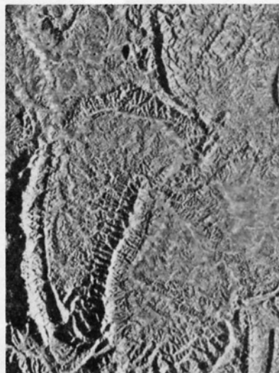
8) Comparison of same-scale (about 1:600,000) radar and map of Monitos rimmed syncline structure in central Sinu Basin. (A) 1969 radar, (B) 1986 airborne radar, and (C) simplified version of photogeologic map. ENE-WSW trending lines in (A) are mosaiced edges of individual flight strips. On map (C), arrows point to trace of significant strike-slip fault and dotted areas are mud volcanoes and/or chaotic zones (interpreted from air photos).
