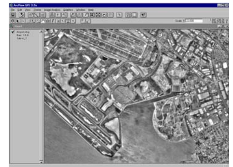
Orthophotography provides a high resolution base with engineering-level x,y accuracy
