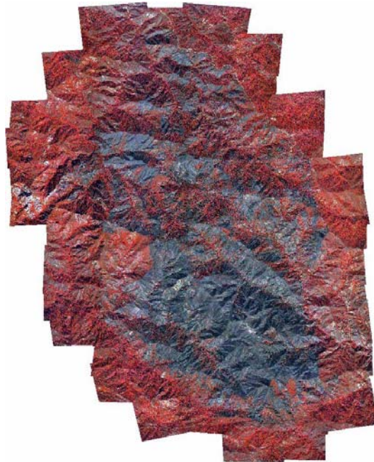
Figure 2. Digital mosaic of ~75 frames of single-camera imagery. Dark area in center is burned forest. GSD = 2 meters. USGS DOQ was the base for georeferencing. Turn-around time <5 days. Imagery acquired with colorIR filter.
