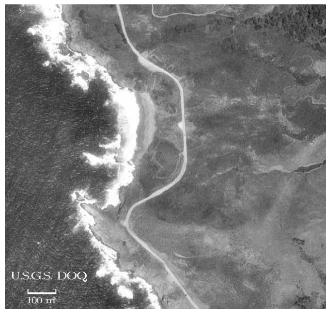
Figure 6. B&W USGS DOQ photograph for comparison to digital frame camera image (Figure 5). The USGS DOQ served as the 1:24,000 base for rectification of new digital color IR imagery.
