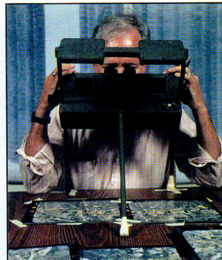
Pat Caldwell, remote sensing analyst for Chevron Overseas Petroleum, Inc., interprets a stereo pair of aerial photographs taken of the Tengiz oil field in Kazakhstan.
