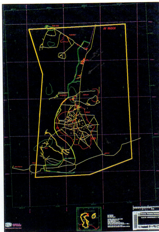
Figure 2: CAD basemap generated from interpretation of satellite images and field work with GPS technology.
